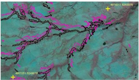
Figure 5. SWF layer originally (magenta) and with corrected projection (black) on Orthophoto (Source MML/Oct2020) in Northern Finland. Coordinates ETRS Laea; scale 1: 70 000.
